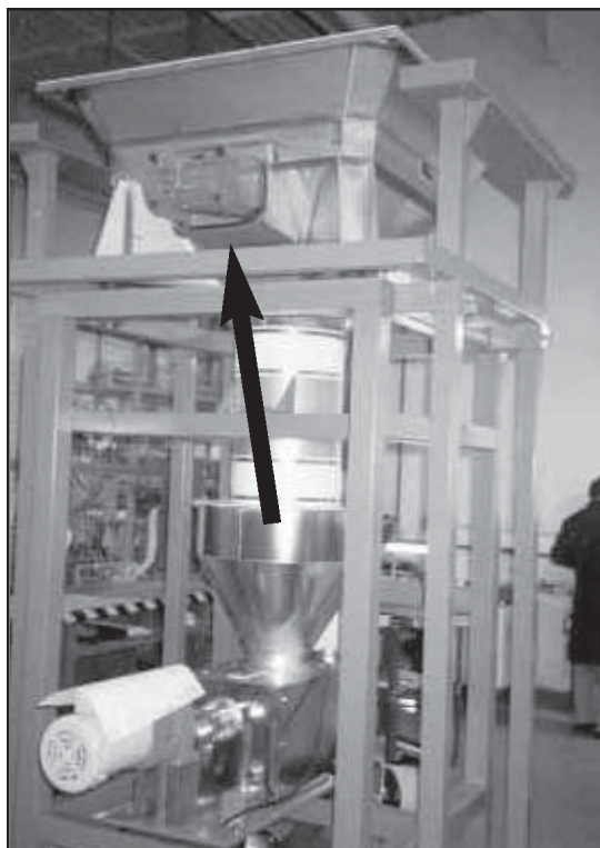
SCR-500 on Box Dumper to prevent hang-ups.
